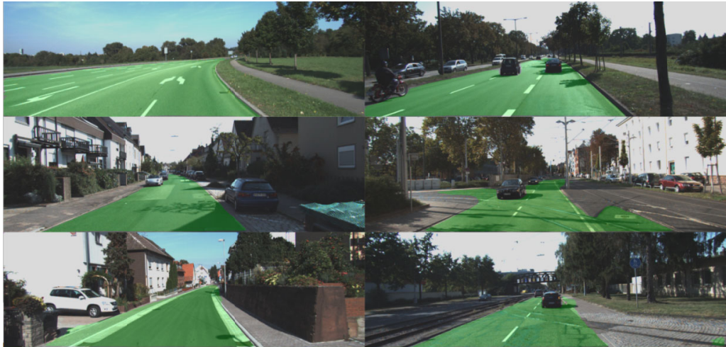
Figure 5. Road sections detected in test images
